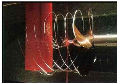
Figure 5, from the Rosi National Laboratory in Denmark, shows the development of the helix from an actual wind turbine using a smoke trace from the tip of one of the three blades. If two wind turbines are close enough in line, it may be possible for the vortices from the blade tips of one to interact with those thrown off by an adjacent one increasing the power of the new vortices and hence the aerodynamic noise produced [Shephard 2010].
