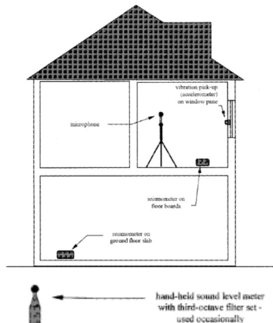
FIGURE 1. Equipment setup<sup>15</sup>
