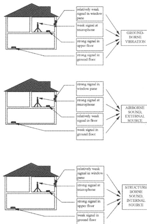
**Figure 2.** Identification of transmission paths and external/internal sources of low frequency noise/vibration<sup>15</sup>
