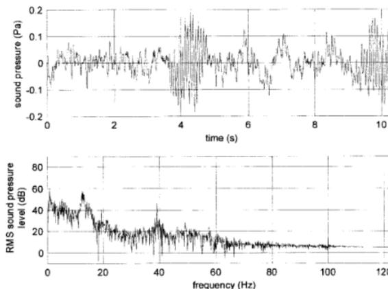
Figure 4. A typical microphone channel recording from H1. From plots such as these, it was possible to identify frequency bands 'of interest' with reference to DIN 45680. Particular focus was given to third-octave bands for which the DIN curve was exceeded and in which the sound displayed an 'unusual' character in the time and/or frequency domains. If both these conditions are met, then low frequency sound can be considered to be potentially annoying according to DIN 45680, as explained earlier.
