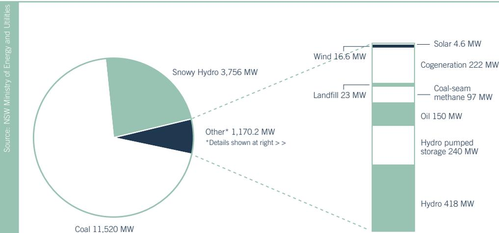
Installed NSW generation capacity by fuel type
