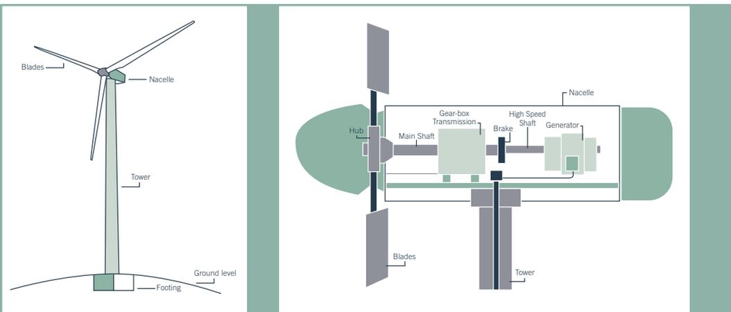
**Nacelle:** Meaning 'small boat' in French, the nacelle sits on top of the tower and houses the gearbox and generator. The hub supporting the blades is attached to it at one end. Nacelles are of varying sizes, depending mainly on the design and size of the generator, and may weigh between 20 and 70 tonnes. The nacelle revolves horizontally on the tower ('yawing') to allow the rotor to face the wind regardless of its direction.
